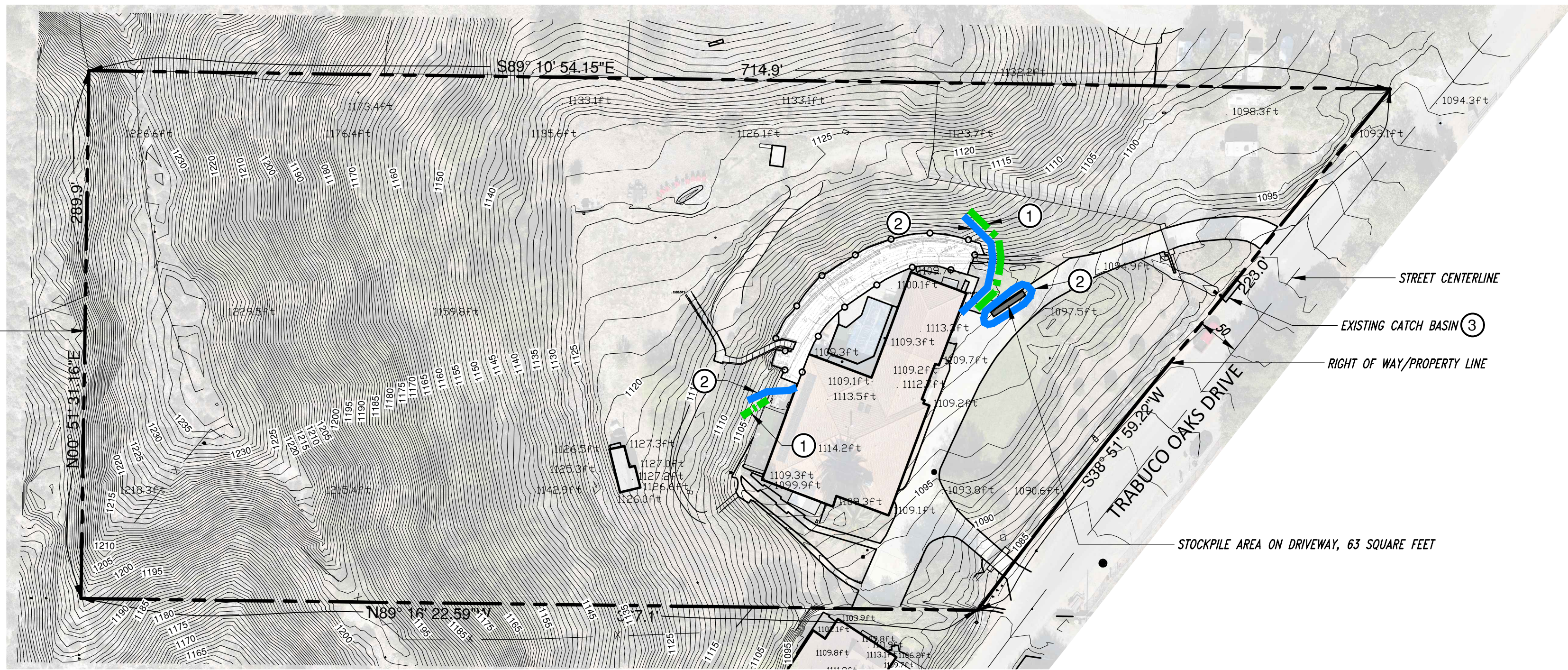
1 EROSION CONTROL PLAN
